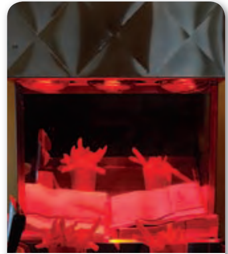
■ Figure 11.6 A heat lamp transfers thermal energy by radiation. Here, the thermal energy helps to keep the french fries hot.
